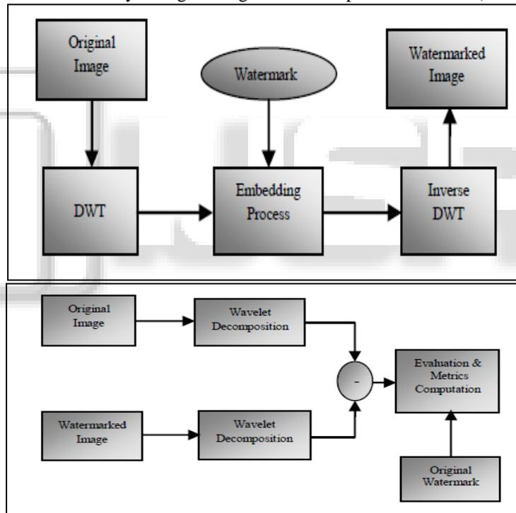
Fig. 1: Image Watermarking Using DWT
