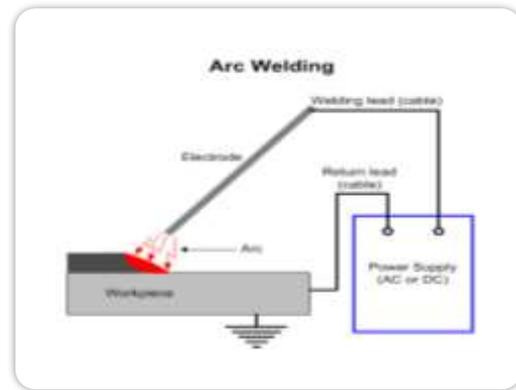
Fig. 11: Arc Welding
