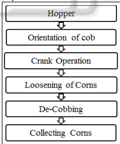
Fig. 4: Flow Diagram
