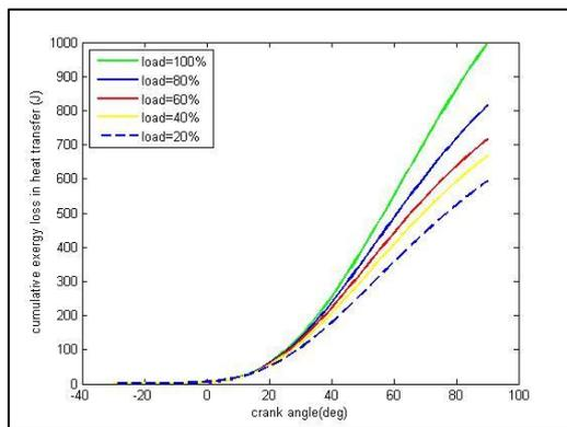
Fig. 6: Cumulative Exergy Loss In Heat Transfer Vs Crank Angle For B10 Biodiesel Fuel
