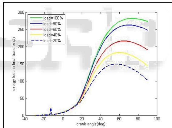
Fig. 5: Exergy Loss In Heat Transfer Vs Crank Angle For B10 Biodiesel Fuel
