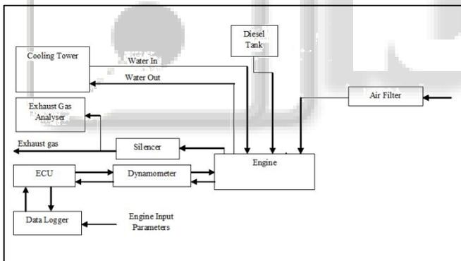
Fig. 1: Engine Setup Block Diagram
