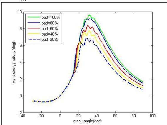
Fig. 3: Work Exergy Rate Vs Crank Angle For B10 Biodiesel Fuel
