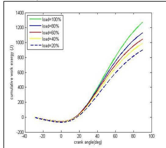
Fig. 4: Cumulative Work Exergy Vs Crank Angle For B10 Biodiesel Fuel
