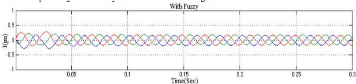
Fig. 8: Current Waveform (With Fuzzy)
