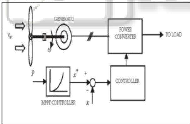
Fig. 4: Block diagram of HCS control
