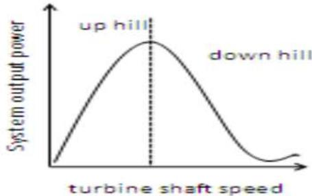
Fig. 3: Principle of Hill-Climb Search control
