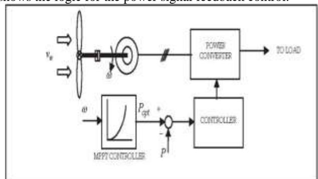
Fig. 2: Block diagram of PSF control
