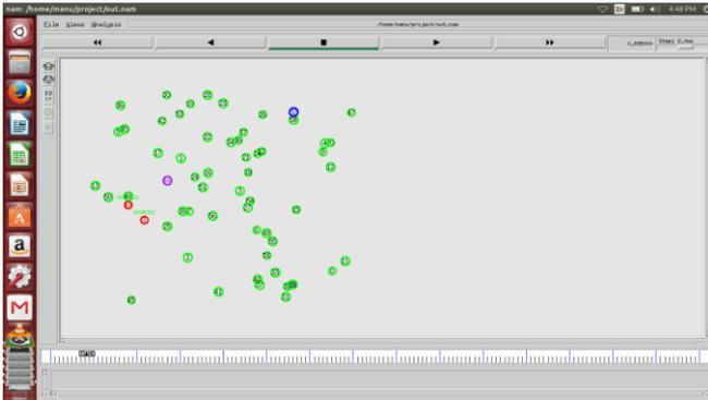
The above window shows the deployment of nodes. When we simulate the network, two nodes were taken as source node1 and source node2 (window source node1 is 8 and source node2 is 13). Node 14 is bottleneck node. Node 32 is destination node or sink node. For every simulation this same process repeats.
