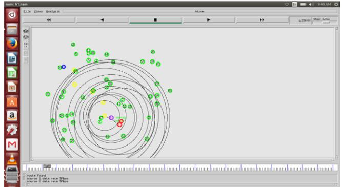
In hybrid technique source nodes send its data to destination through a bottleneck node or intermediate node. If congestion is seen at bottleneck node then it will send a back pressure message to a source node then source node reduces its data rate and at the same time it will look for alternate path to send its data. This improves the quality of service (QoS) and time delay. We are giving knowledge to a node whether it should apply for a traffic control or a resource control.
