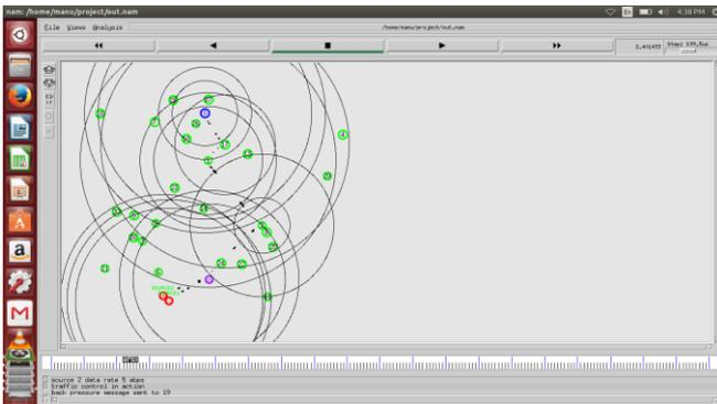
The above window shows the simulation of Traffic control algorithm with transferring packets from source node to sink node. Source node data rate decreased and avoiding congestion. Source node chooses the path towards sink node randomly in the direction of destination node. The above window shows path with packets transmission
