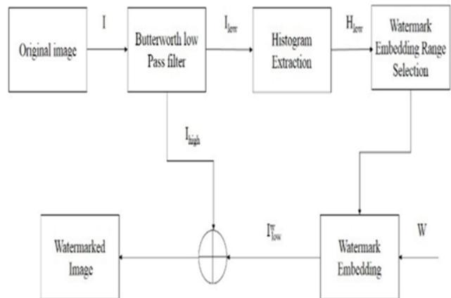
Fig. 2: Block Diagram of Watermark Embedding Process
