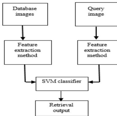
Fig. 1: block diagram of CBIR
