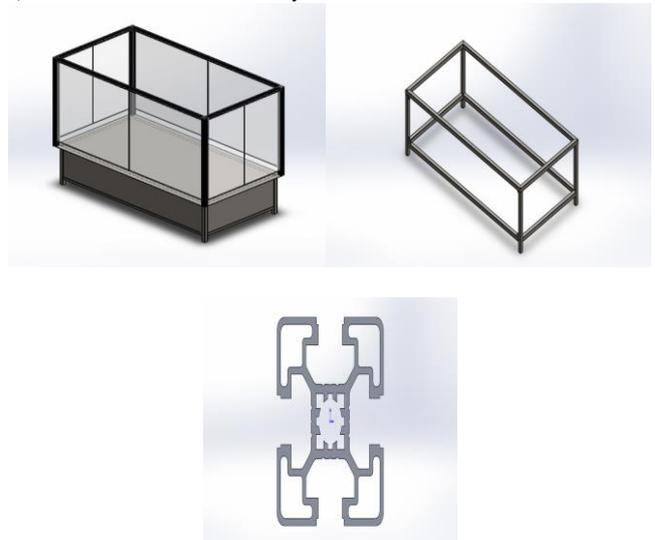
The structure assembly contains the guard plate which is made up of AISI 1035 structural steel. The thickness of the plate is 1.2mm and bend radius is 0.7366 mm and the size of the plate is 919mm x 469 mm. The no of quantity are four.
