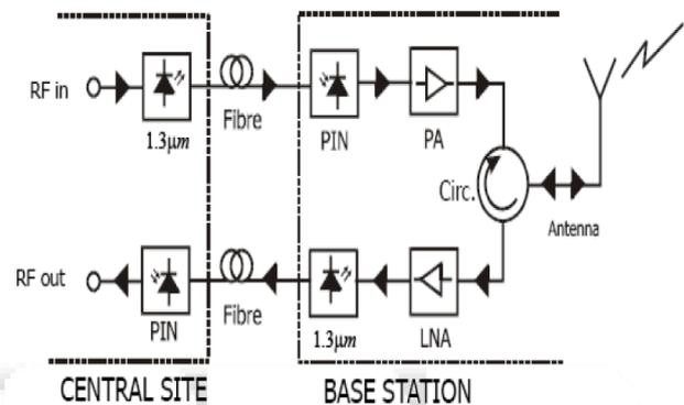
Fig. 1: Radio on Fiber System
