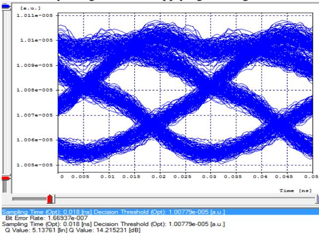
By comparison of both eye diagram it is clear that by applying appropriate filtering action Q-factor of signal
