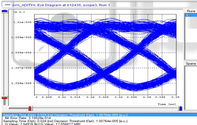
Eye diagram before applying filtering action
