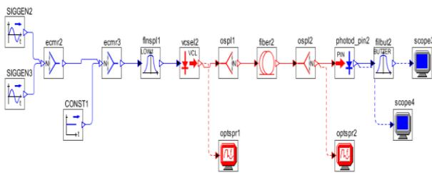
Fig. 3: Direct Modulation Through VCSELs
