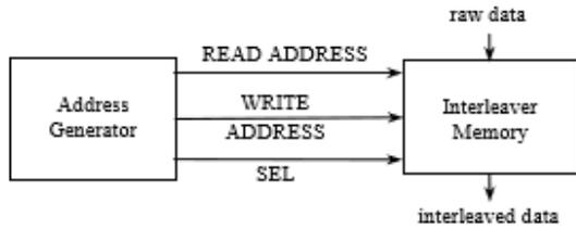
Fig. 2: Top level view of WiMAX interleaver
