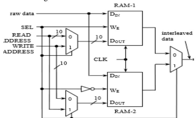
Fig 4: schematic view of interleaver memory block
