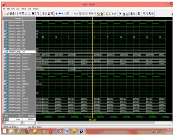
Fig. 5: simulation results for BPSK
