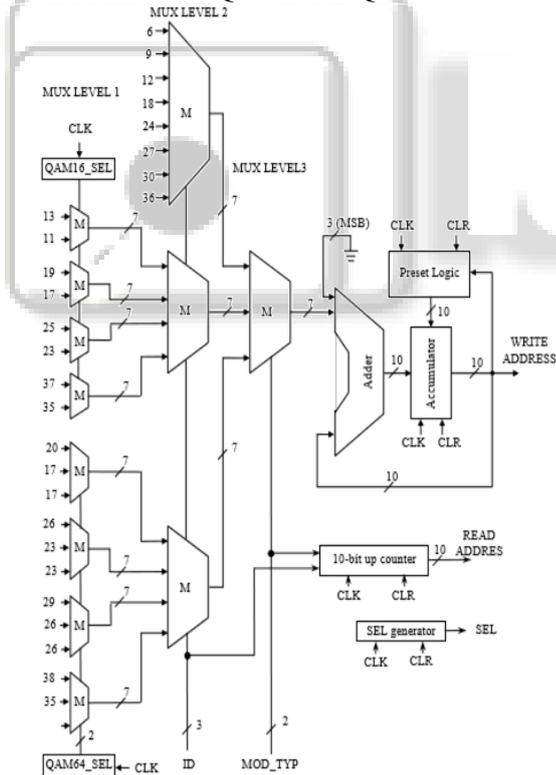
Fig. 3: Address generator of interleaver
