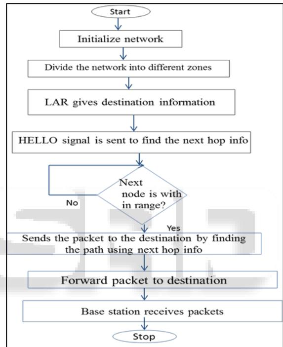
Fig. 2: Flow Chart for Routing
