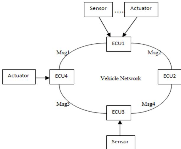
Fig. 1: Iner ECU Communication
