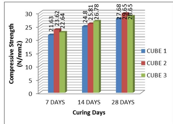
Fig. 4: Chart for Compressive Strength of MIXES 3 Cubes
