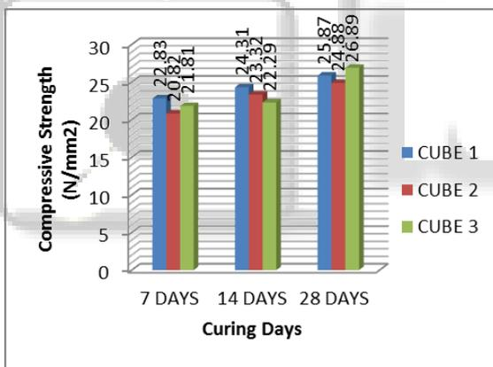
Fig. 3: Chart for Compressive Strength MIX 2 Cubes
