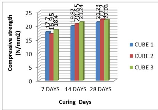
Fig. 2: Chart For Compressive Strength of MIX 1 Cubes
