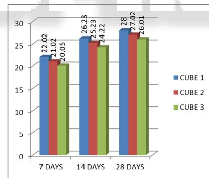
Figure 5: Chart for Compressive Strength of MIX 4 Cubes
