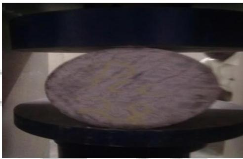
Fig. 7: Split Tensile Strength Test for Cylinder
