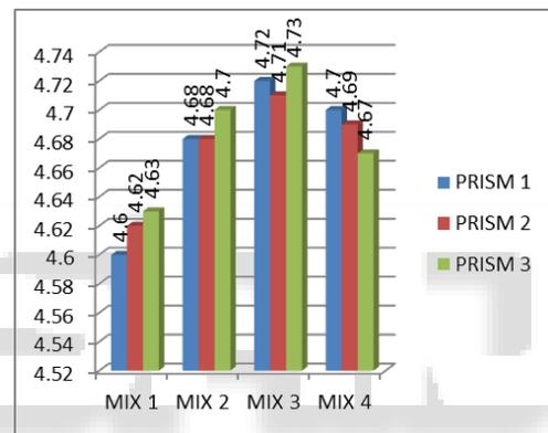
Fig. 10: Chart for Flexural Strength of Various Mix of Prisms
