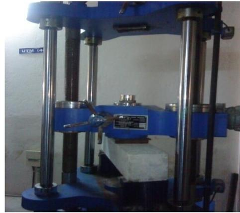
Fig. 9: Flexural Strength Test for Prism
