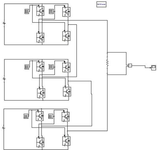
Fig. 4: Schematic of Conventional Seven Level Inverter
