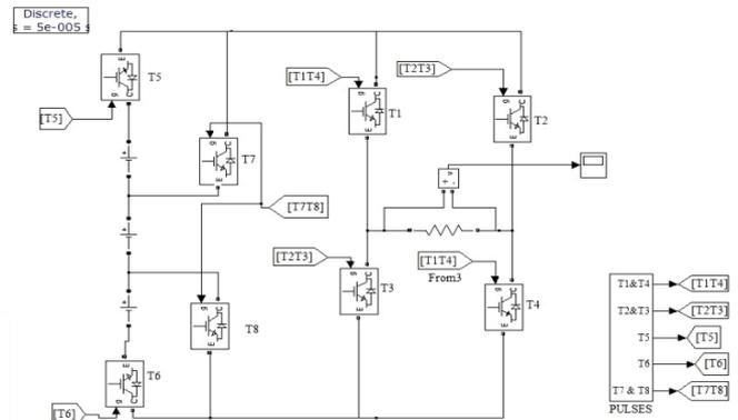
Fig. 5: Schematic of conventional Seven Level Inverter
