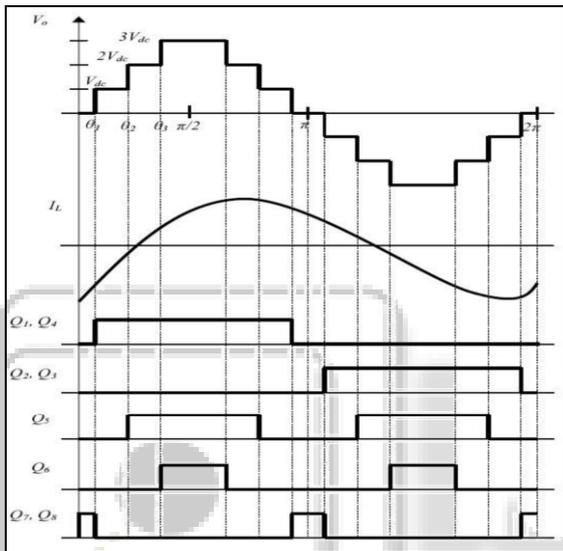
Fig. 3: Waveforms of the Proposed 7-Level Inverter
