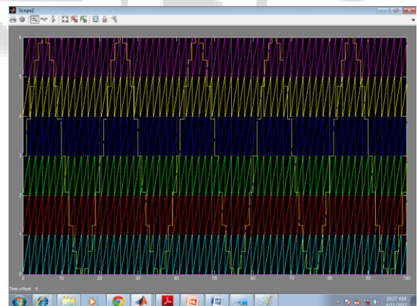
Fig. 6: Six Different Levels Of Saw Tooth Carrier Signal Compared With Digital Sinusoidal Counter Based Signal.
