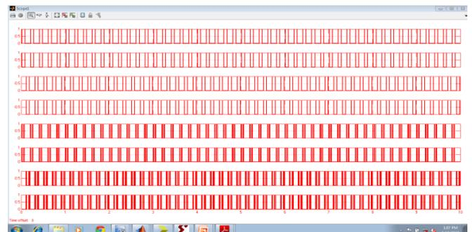
Fig. 7: Switching Pattern of Single Phase Seven Level Inverter Topology
