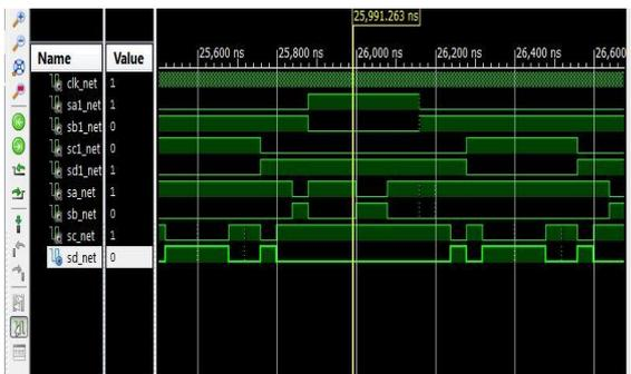
Fig. 8: DPWM Signal In Xilinx System Generator
