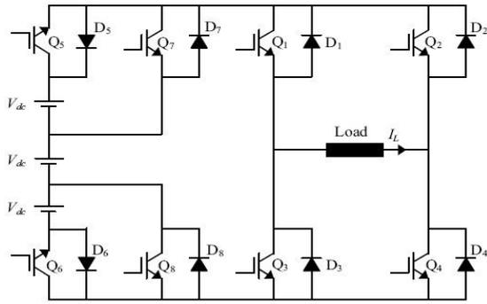
Fig. 2: The 7-Level Inverter of the New Topology
