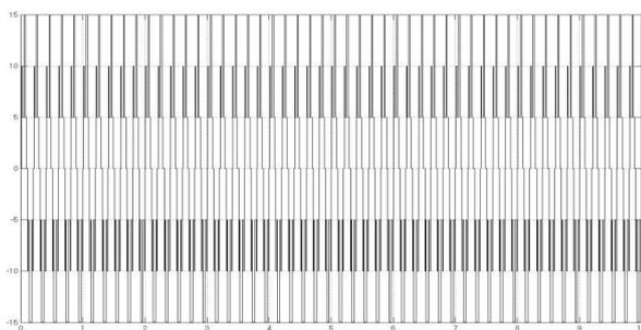
Fig. 9: Output Voltage for Single Phase Seven Level Inverter
