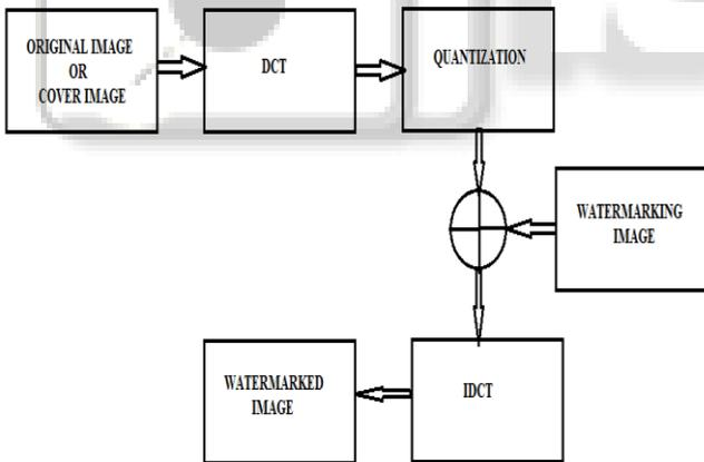
Fig. 1: Block Diagram of Watermark Embedding
