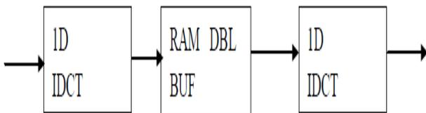
Fig. 4: 2D-IDCT Using Vector Processing
