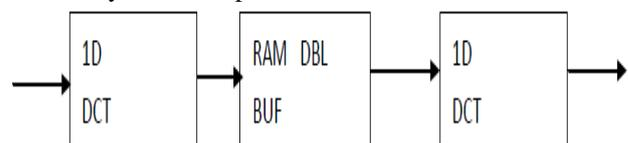
Fig. 3: 2D-DCT Using Vector Processing
