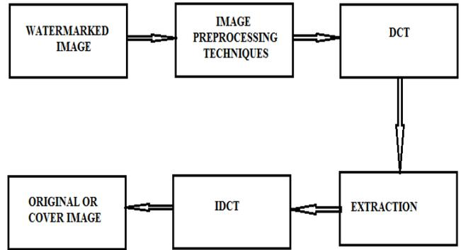
Fig. 2: Block Diagram of Watermark Extraction
