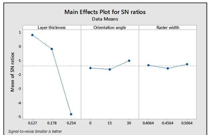
Fig. 6: Main Effect Plot (C) Percentage Change In Thickness For S/N Ratio (Smaller Is Better)
