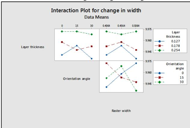
Fig. 8: Interaction Plot Of Every Parameter With Each Other For Percentage Change In Width
