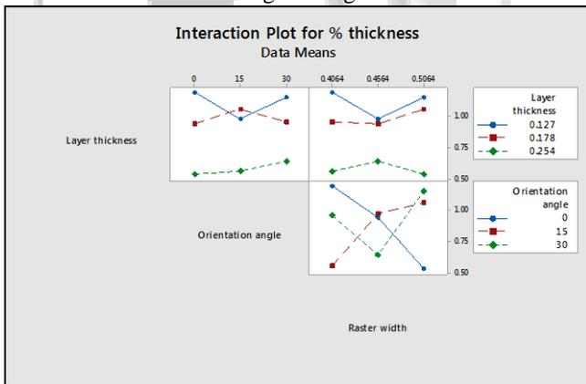
Fig. 9: Interaction Plot of Every Parameter with Each Other For Percentage Change in Thickness
