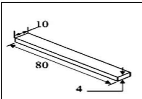
Fig. 3: Specimen Design for Dimensional Accuracy
