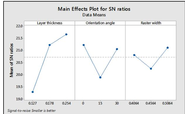
Fig. 4: Main Effect Plot (A) Percentage Change In Length, For S/N Ratio (Smaller Is Better)
