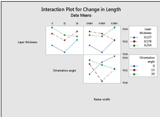
Fig. 7: Interaction Plot of Every Parameter with Each Other For Percentage Change in Length
