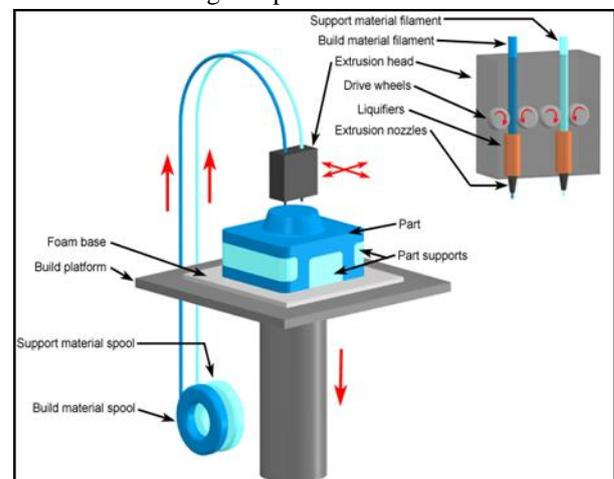
Fig. 1: Fused Deposition Modeling (FDM)<sup>[4]</sup>
