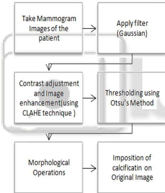
Fig. 4: Flow of Implementation for Detection of Micricalcification
