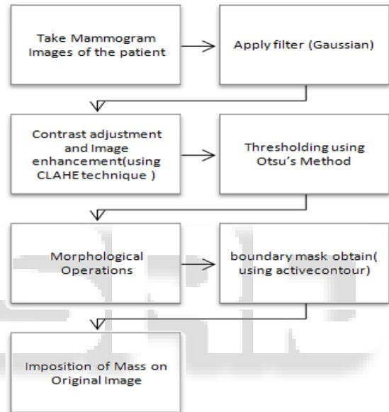
Fig. 6: Flow of Implementation for Detection of Mass
