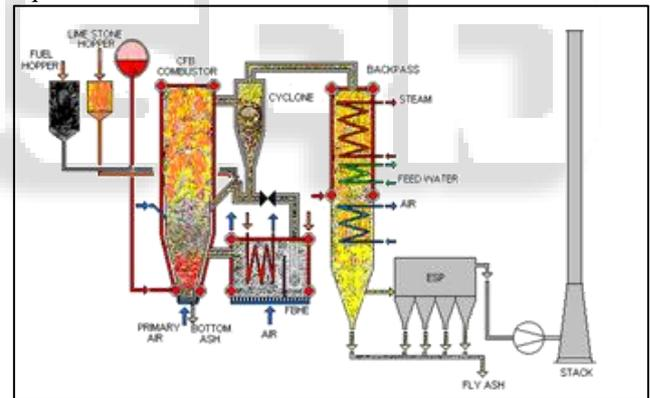
Fig. 3: Schematic of a Circulating Fluidized Bed Combustion Boiler
