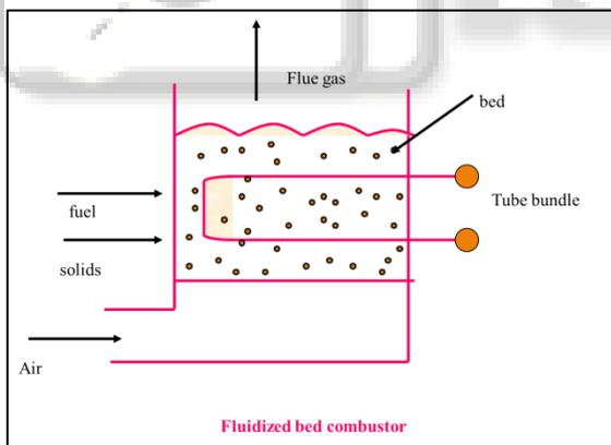
Fig. 2: Schematic of Fluidization Bed
