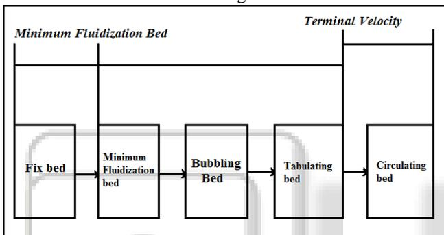
Fig. 1: Flow Diagram of Fluidization of Bed with Increase in Air Velocity
