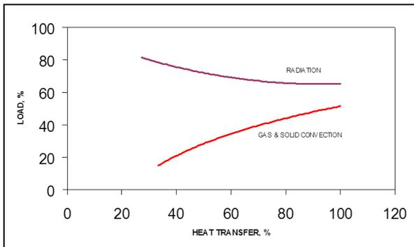
Fig. 7: Effect of Load Reduction on Heat Transfer Components
