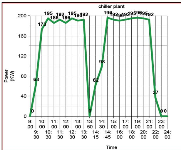
Fig. 4: Cold Load Pickup Curve For Chiller Plant
