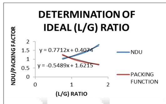
Fig. 8: (NDU) and Packing Function Versus (L/G) Ratio
