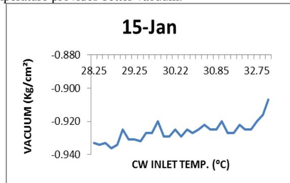
Fig. 5: Vacuum Variation with Inlet Cooling Water Temperature.
