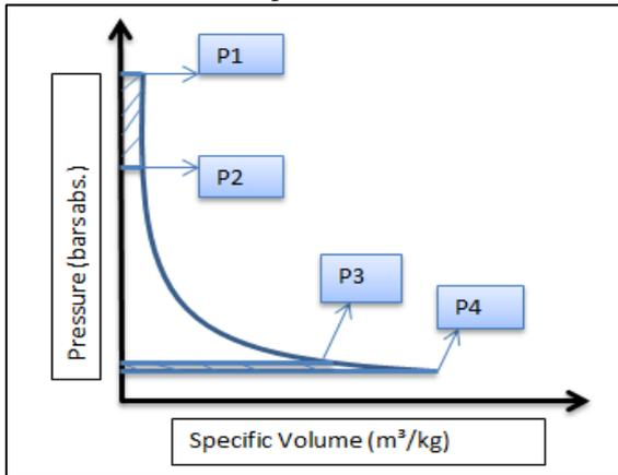
Fig. 2: Pressure v/s Specific Volume for Dry Saturated Steam
