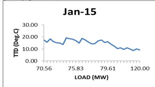
Fig. 6: Terminal Temperature Difference (TTD) Variation with Load.
