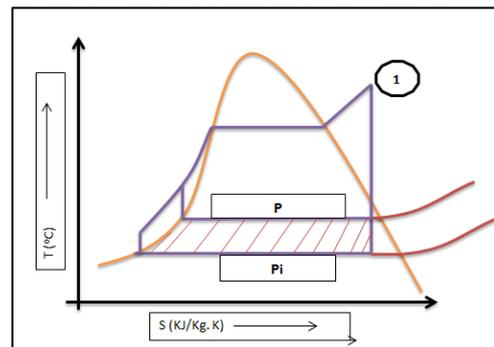
Fig. 1: Effect of Improving the Condenser Vacuum
