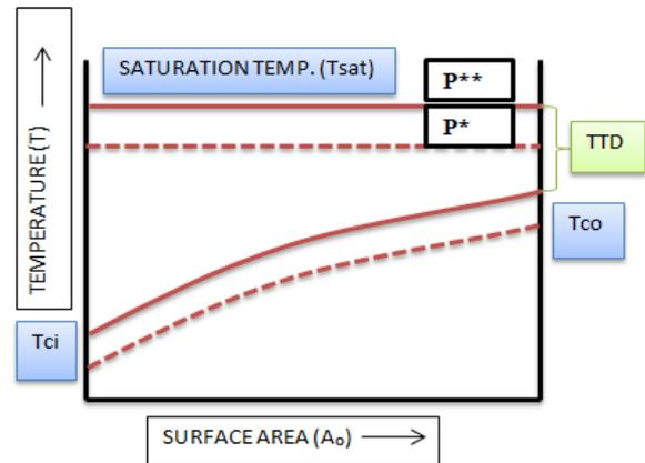
Fig. 4: Change in Vacuum Pressure with Change in Inlet CW Water Temperature.
