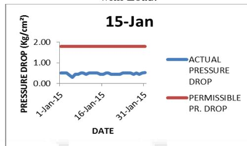
Fig. 7: Pressure Drop Variation with Time
