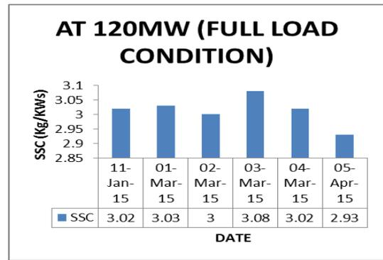
Fig. 3: Specific Steam Consumption V/S Time.
