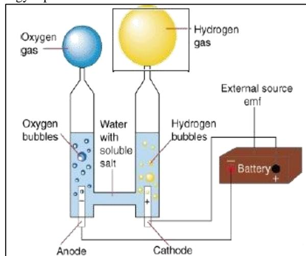
Fig. 5: Electrolysis of Water
