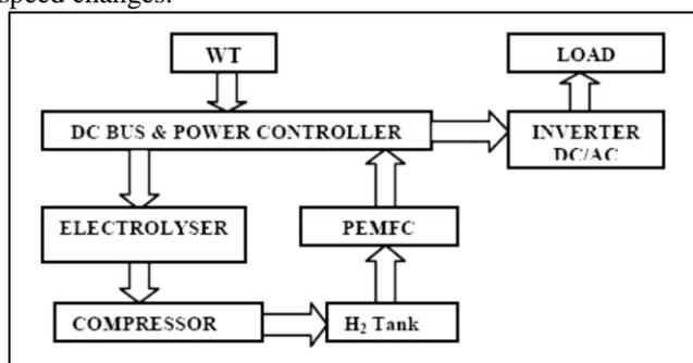
Fig. 9: Hybrid Wind- Hydrogen System Diagram
