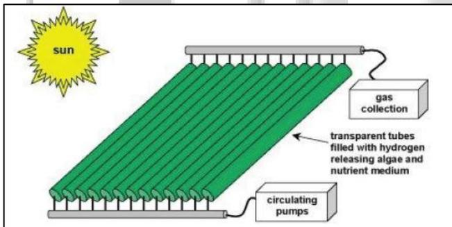
Fig. 7: Hydrogen Production from Algae by Using Solar Energy
