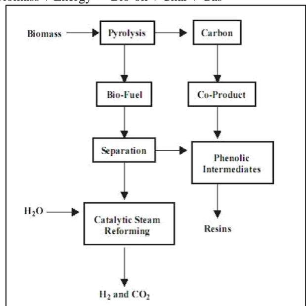
Fig. 8: Pyrolysis Process For Hydrogen Production
