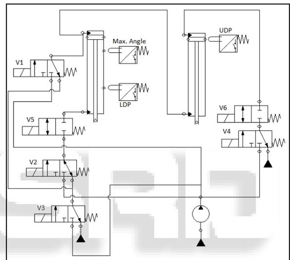
Fig. 7: Mechanism for Executing Stroke and Angle Change
