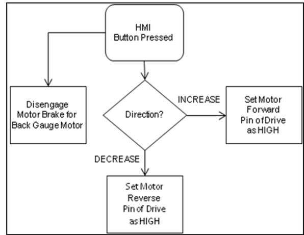
Fig. 6: Back Gauge Motor Logic
