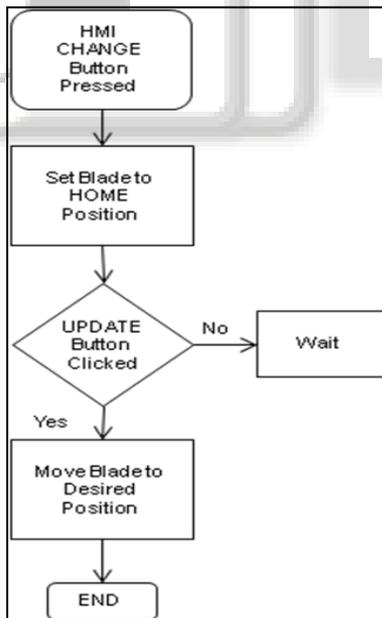
Fig. 5: Blade Clearance Updation Logic
