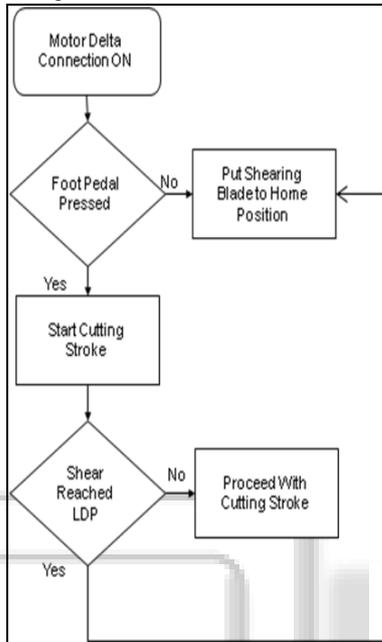
Fig. 4: Stroke Logic
