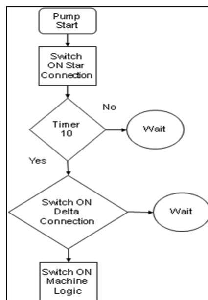
Fig. 3: Machine Start-Up Logic
