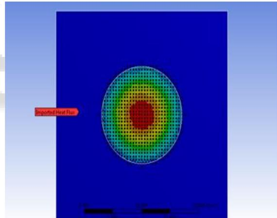
Fig. 1.4: Output of Gaussian load on front of rectangular plate with source data
