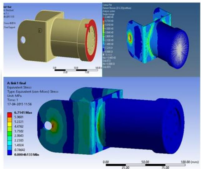
Fig. 4: Loading condition, Equivalent stress value in Hypermesh and Workbench (6.5MPa, F.O.S 44)
