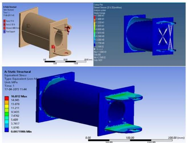
Fig. 5: Loading condition, Equivalent stress value in Hypermesh and Workbench (16 MPa, F.O.S 18)
