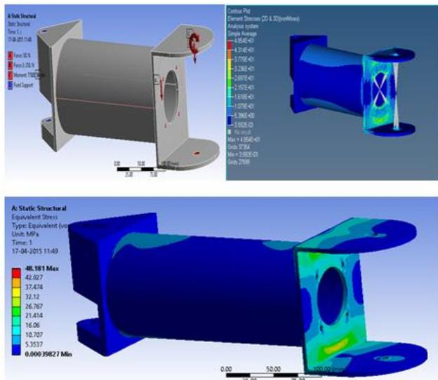
Fig. 7: Loading condition, Equivalent stress value in Hypermesh and Workbench (48MPa, F.O.S 5)
