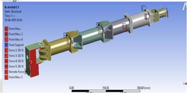
Fig. 10: boundary condition for fully stretch condition
