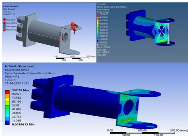
Fig. 8: Loading condition, Equivalent stress value in Hypermesh and Workbench (102 MPa, F.O.S 2.84)
