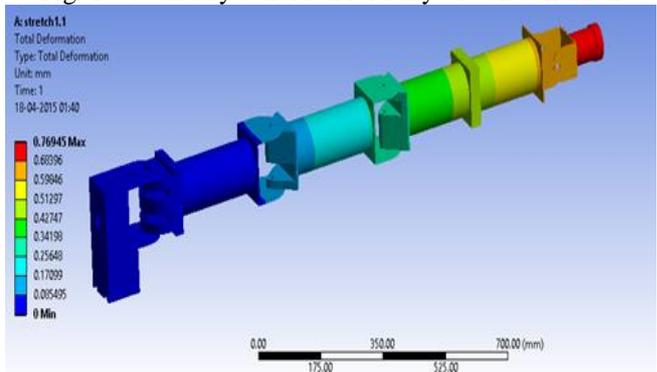
Fig. 11: Total deflection in stretch condition 0.76 mm
