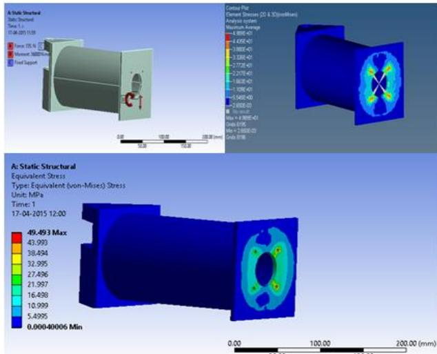
Fig. 6: Loading condition, Equivalent stress value in Hypermesh and Workbench (49 MPa, F.O.S 5)
