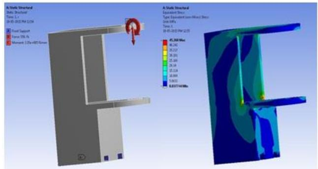
Fig. 9: Loading condition, Equivalent stress value in Hypermesh and Workbench (45 MPa, F.O.S 5)
