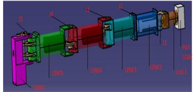
Fig. 1: Proposed design of articulated robot arm
