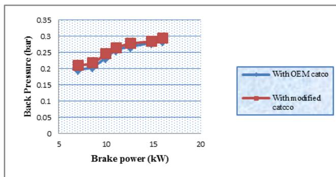
Fig. 8: Back Pressure Vs Brake Power:
