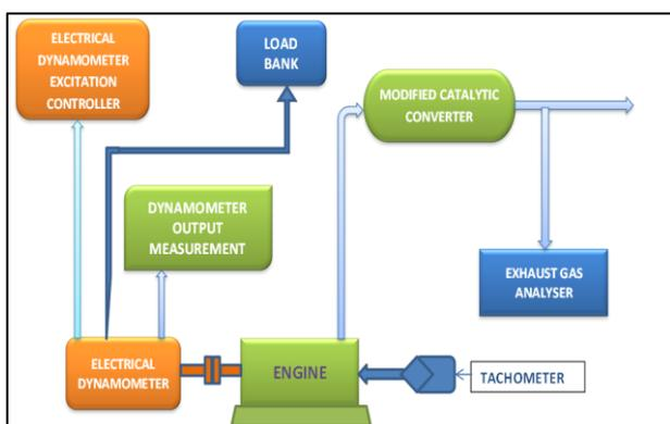
Fig. 3: Layout of Experimental Setup
