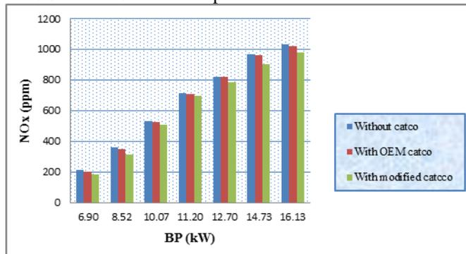
Fig. 6:  $\text{NO}_x$  Vs Brake Power
