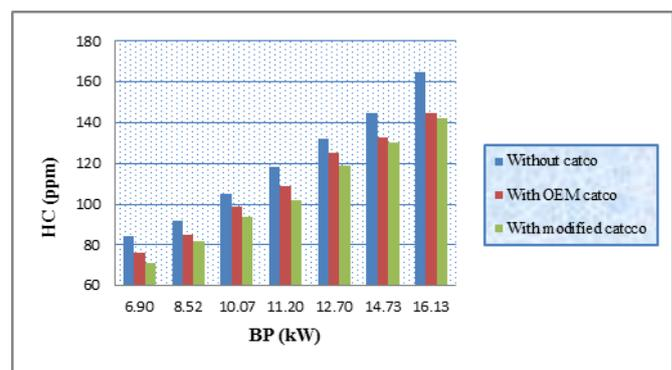
Fig. 5: HC Vs Brake Power:
