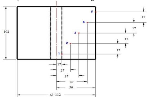
Fig. 2: locations of the different thermocouples
