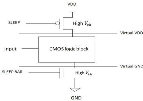
Fig. 1: structure of Multi Threshold CMOS
