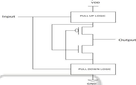
Fig. 6: leakage control transistor
