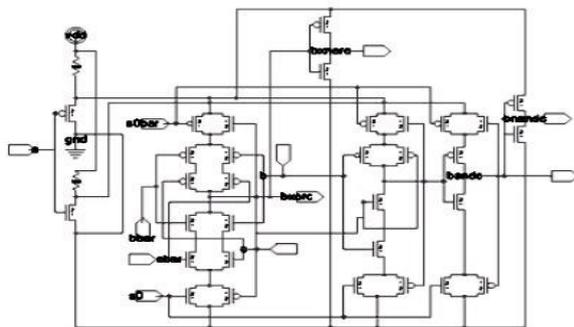
Fig. 7: full adder with sleepy keeper
