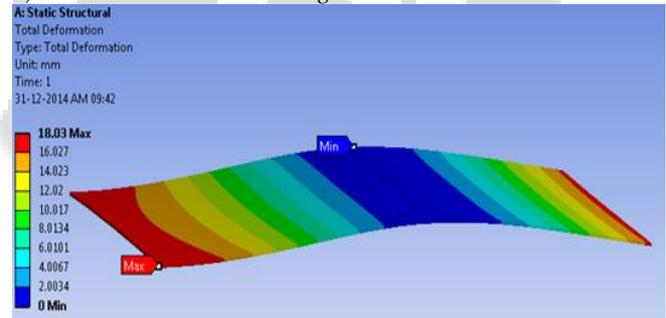
Fig. 3: Deformation in 10meter plate
