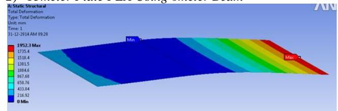
Fig. 5: Deformation in 13meter plate
