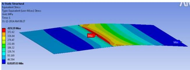
Fig. 6: Stress in 13meter plate
