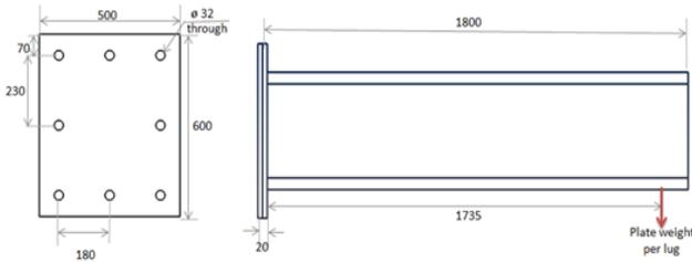
Direct shear load on each bolt
