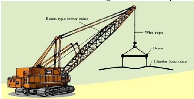
Fig. 2: 6meter beam lifting 13 meter plate
