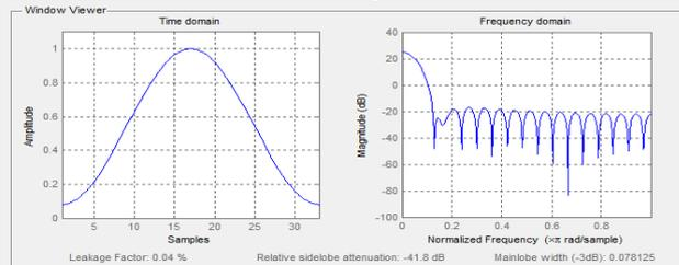
Low Pass Filter Using Hamming Window
