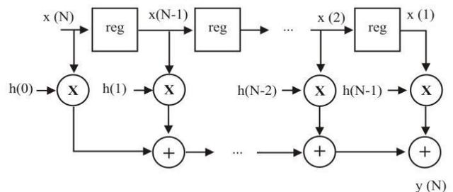
Fig. 2: Direct Form Realization Structure Of An FIR System.
