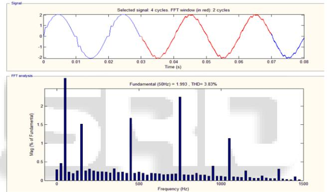
Fig. 9: THD% analysis with Configuration 1 Hybrid Filter with unbalance load
