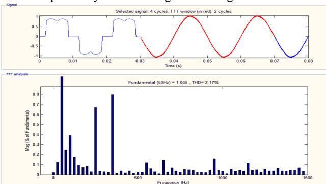
Fig. 14 THD% analysis with Configuration 3 Hybrid Filter with balance load
