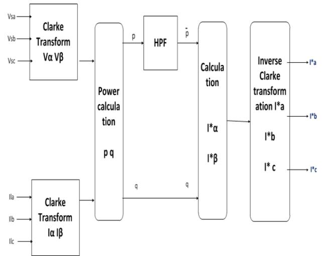
Fig. 4: Block diagram of Instantaneous reactive power theory
