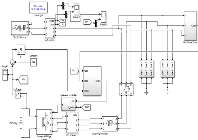
Fig. 5: Simulation model of Hybrid Active Filter configuration 1
