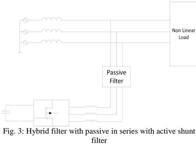
Fig. 3: Hybrid filter with passive in series with active shunt filter
