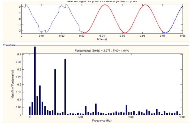
Fig. 8: THD% analysis with Configuration 1 Hybrid Filter with balance load
