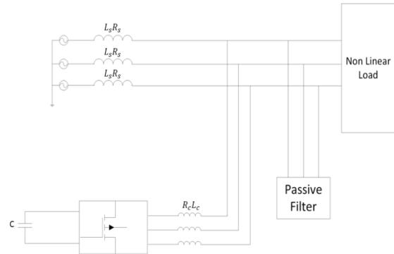
Fig. 1: Hybrid filter with active and passive both in shunt Active filter. This will make both active and passive filters overloaded
