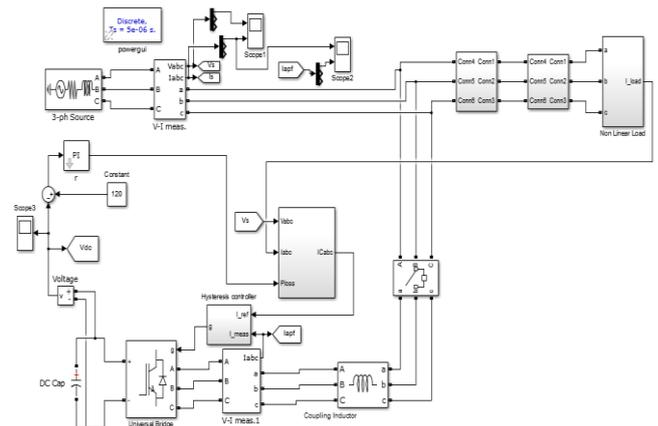
Fig. 10: Simulation model of Hybrid Active Filter configuration 2
