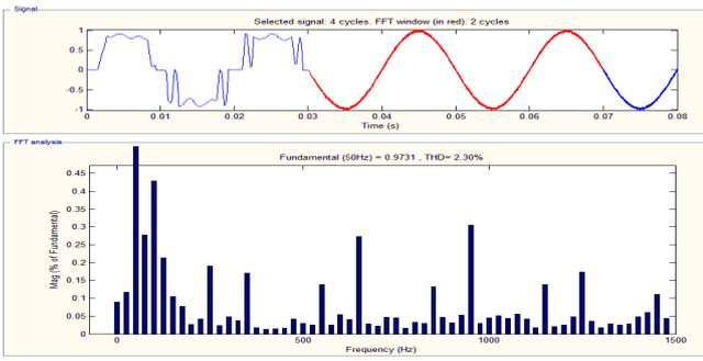
Fig.11: THD% analysis with Configuration 2 Hybrid Filter with balance load
