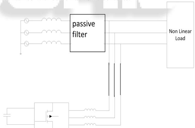
Fig. 2: Hybrid filter with active in shunt and passive in series
