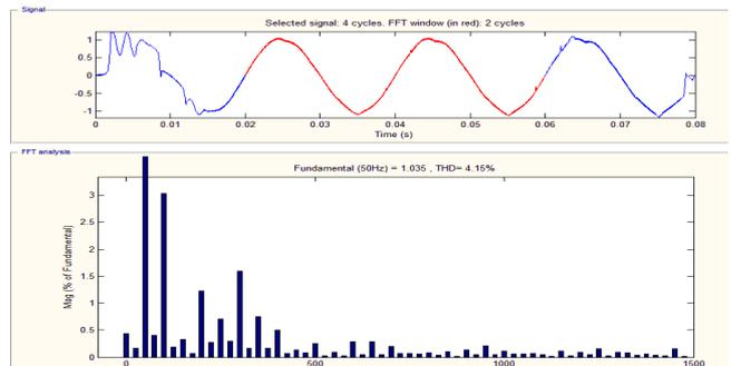
Fig. 15 THD% analysis with Configuration 3 Hybrid Filter with unbalance load
