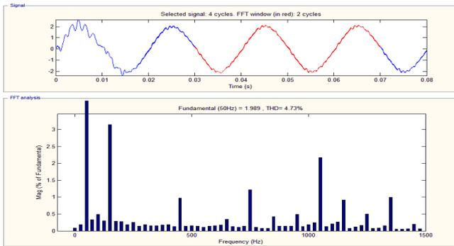
Fig.12 THD% analysis with Configuration 2 Hybrid Filter with unbalance load
