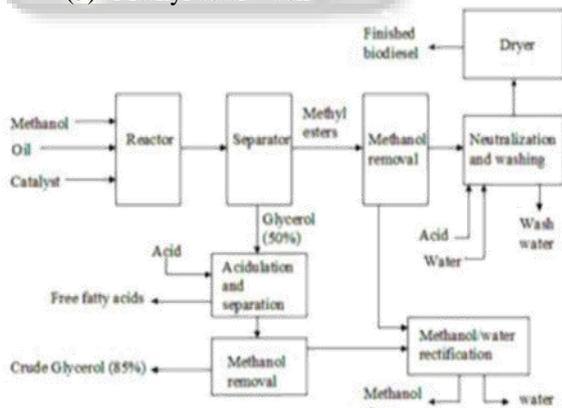
Fig. 1: Production Process of Biodiesel
