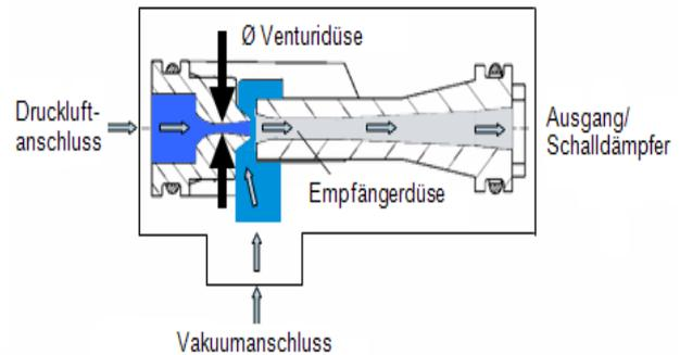
Fig. 2: The Operation Of A Venturi
