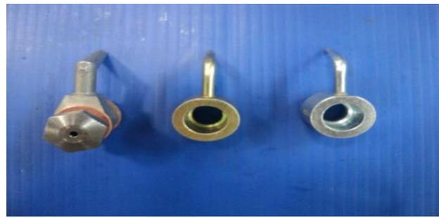
Fig. 9: Piston Cooling Nozzle
