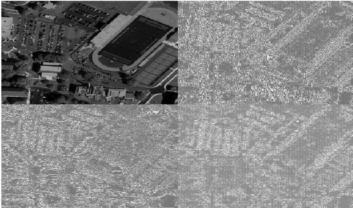
Fig. 3: LL, LH, HL, and HH Subbands of a Satellite Image Obtained By Using DWT.
