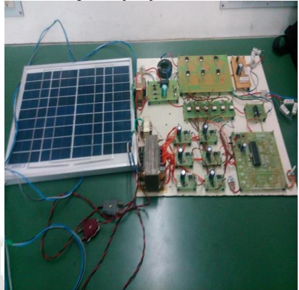
Fig. 5: Photograph of the MOSFET-based laboratory prototype of the BDHC.
