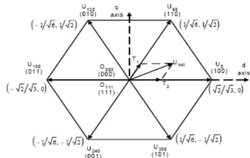
Fig. 3: The Basic Space Vectors (Normalized w.r.t.  $V_{dc}$ ) and Switching States
