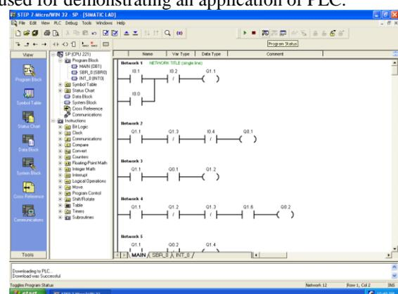
Fig. 3 (A): Ladder Logic for Sequential Batch Process
