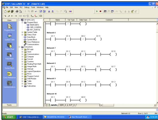
Fig. 3 (B): Ladder Logic of Batch Process
