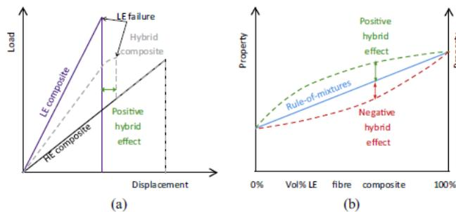
Fig. 2.10: Illustration of the definitions of the hybrid effect: (a) the apparent failure strain enhancement of the LE fibers, under the assumption that relative volume fraction is 50/50 and that the hybrid composite is twice as thick as the reference composites and (b) a deviation from the rule of mixtures. (For interpretation of the references to color in this figure legend, the reader is referred to the web version of this article.)
