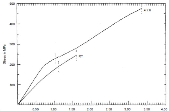
Fig. 2.6: Stress/strain curves for composite material (type U11) at RT and 4.2 K
