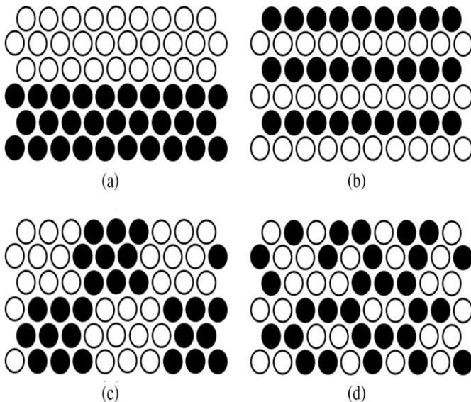
Fig. 2.9: Illustration of the various degrees of dispersion (a) two layers, (b) alternating layers, (c) bundle-by-bundle dispersion, and (d) completely random dispersion.
