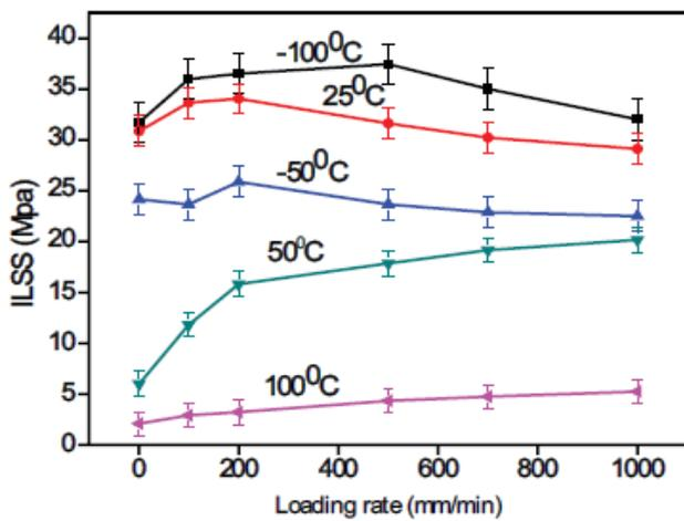
Fig. 2.3: variation of interlaminar shear strength with different loading rates at different temperatures for carbon fibre/epoxy composite system.
