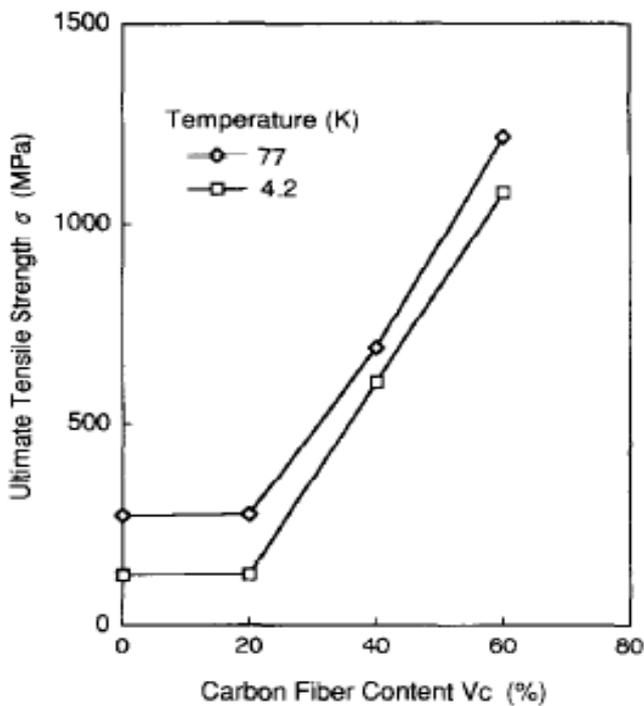
Fig. 2.7: Change in the ultimate tensile strength of CFRP with carbon-fiber content
