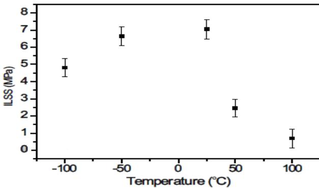
Fig. 2.5: Interlaminar shear strength of Carbon/epoxy composite at 1 mm/min for different temperature.
