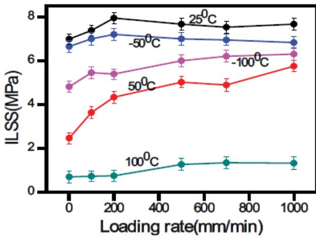
Fig. 2.4: Variation of ILSS with loading rate for Kevlar/epoxy composite system at various temperatures and loading rates.
