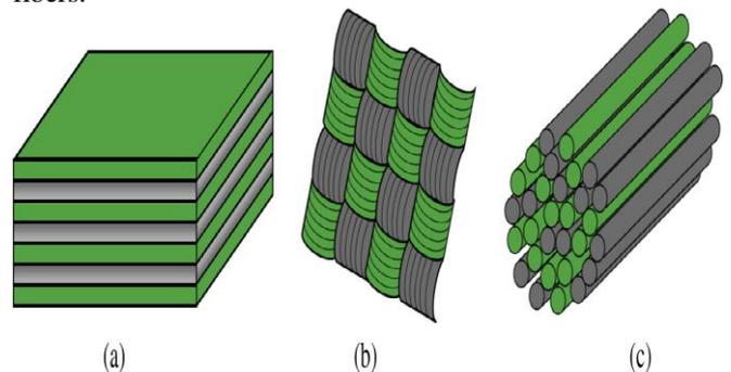
Fig. 2.8: The three main hybrid configurations: (a) interlayer or layer-by-layer, (b) intralayer or yarn-by-yarn, and (c) intrayarn or fibre-by-fibre. (For interpretation of the references to color in this figure legend, the reader is referred to the web version of this article.)
