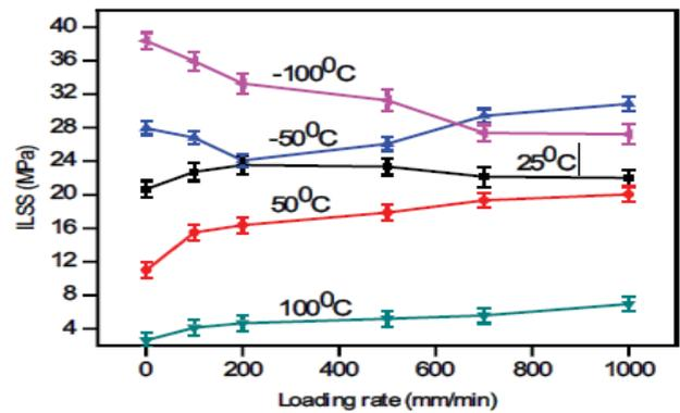
Fig. 2.1: Variation of ILSS with loading rate for glass/epoxy composite system at different temperatures.
