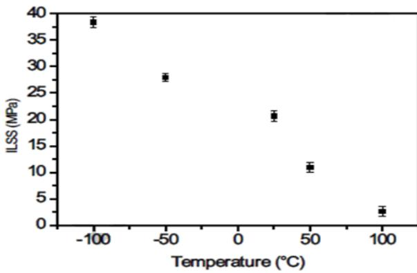
Fig. 2.2: Interlaminar shear strength of glass/epoxy composite at 1 mm/min for different temperature.
