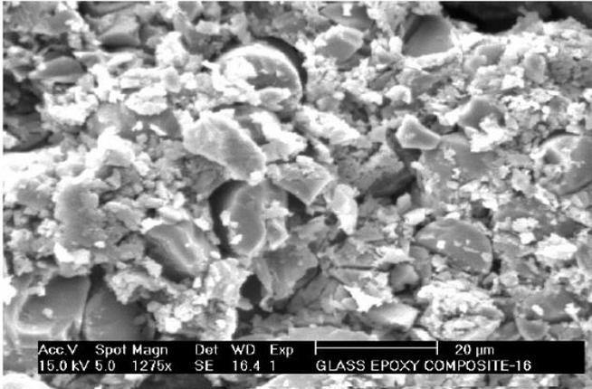
Fig.2.11: Schematic of Matrix cracking at cryogenic temperature i.e.77K.
