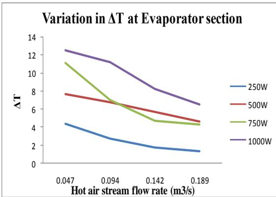
Fig. 4: Variation in  $\Delta T$  at Evaporator Section
