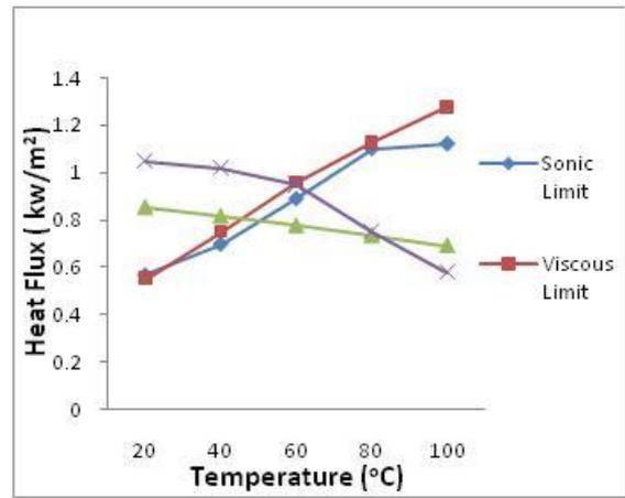
Fig. 3: Heat Pipes Limits for Various Operating Temperatures
