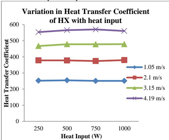
Fig. 10: Variation in Heat Transfer Coefficient of HX with Heat Input
