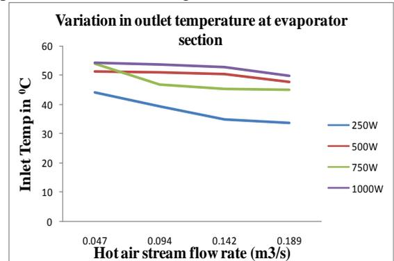
Fig. 7: Variation in Outlet Temperature at Evaporator Section
