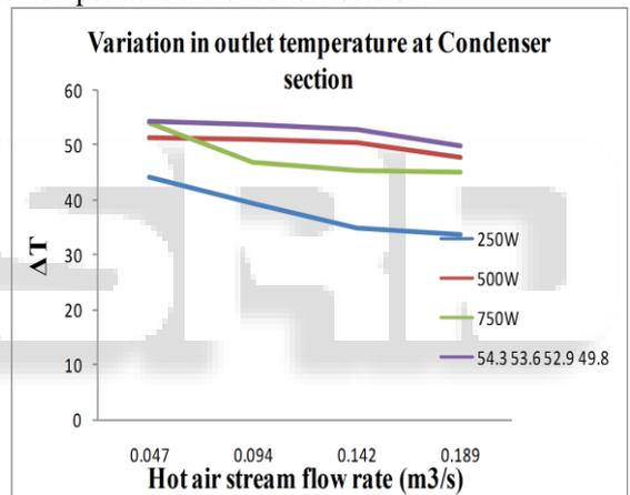
Fig. 8: Variation in Outlet Temperature at Condenser Section
