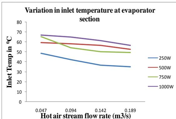
Fig. 6: Variation in Inlet Temperature at Evaporator Section Variation in outlet temperature of evaporator section is observed due to the absorption of the heat by heat pipe working fluid during the phase change. At evaporator section working fluid absorbs the heat and it gets evaporated. So at the outlet of evaporation section temperature decrease and Figure 07 shows the variations.
