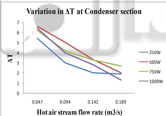
Fig. 5: Variation in  $\Delta T$  at Condenser Section
