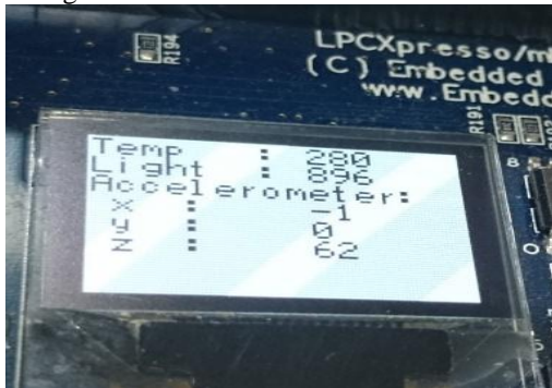
Fig. 5: Sensor Data Displayed on An OLED
