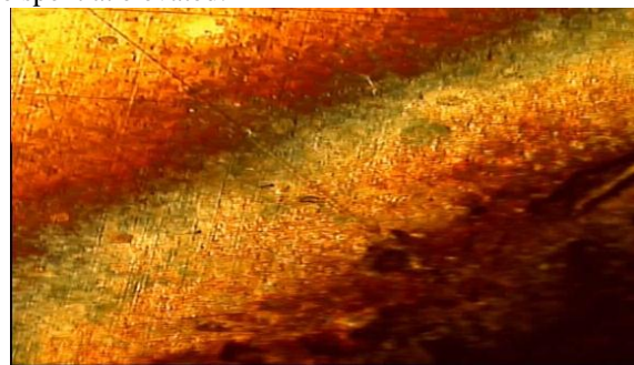
Fig. 3: (100 x) H.A.Z. of a ASS 202-ASS 202- 202- 45 N Electrode force before breaking of nugget
