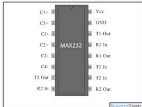
Fig. 2: MAX 232 pin diagram
