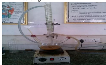
Fig. 2.1(a): Mahua Seed Oil Heating With Reactants in a Three Neck Flask
