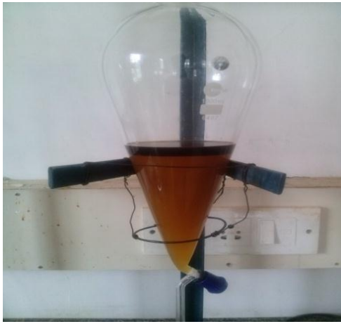
Fig. 2.1(b): FFA and other Impurities Separated from Oil After 1 st Stage of Transesterification
