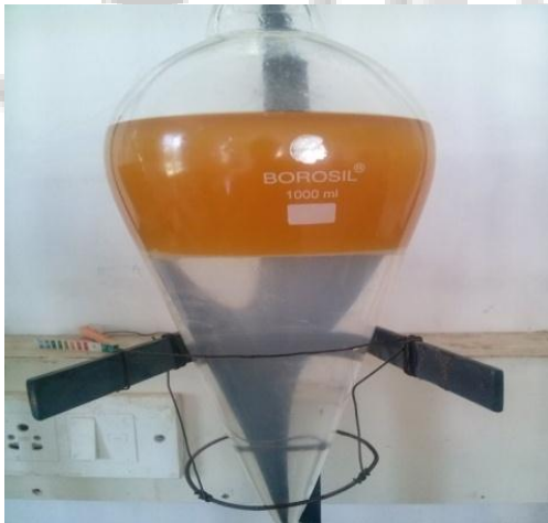
Fig. 2.3: The Separated Glycerol and Water Washed Esters in Separating Flask
