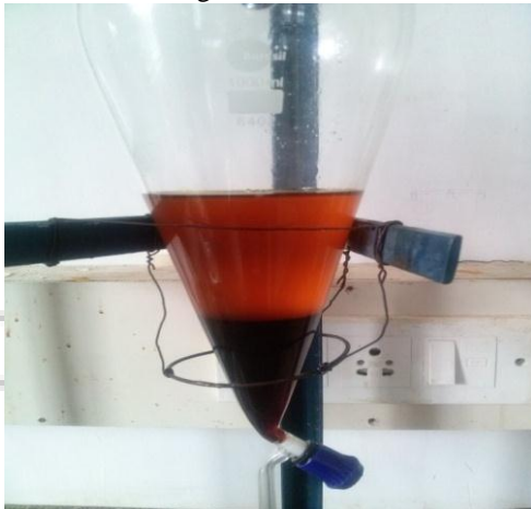
Fig. 2.2: Glycerol Settling After the Stage of Transesterification
