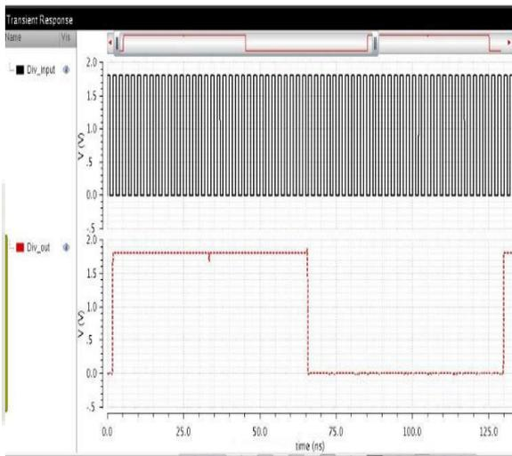
Fig. 13: Output of Divide by 64 Counters
