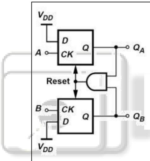
Fig. 2: PFD Schematic Circuit
