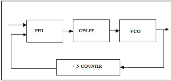
Fig. 1: Block diagram of the proposed PLL.
