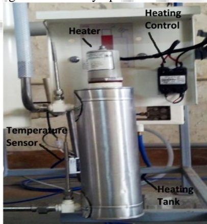
Fig. 1: Heating System Arrangement
