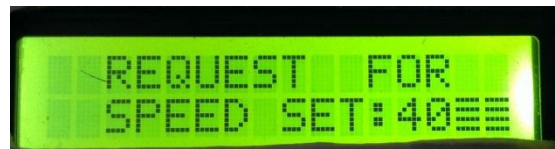
Fig. 12: LCD Showing the Speed Set Dynamically to 40 as Threshold
