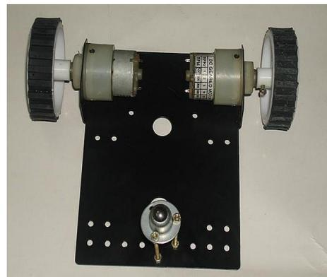
Fig. 4: Wheel Size of 6cm, Chase Height 12\*8cm
