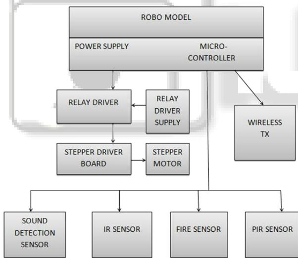
Fig. 2: Block Diagram on Robotic Side
