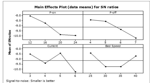
Fig. 13: Effect of Process parameters on Surface Roughness for 16MnCr5 material.
