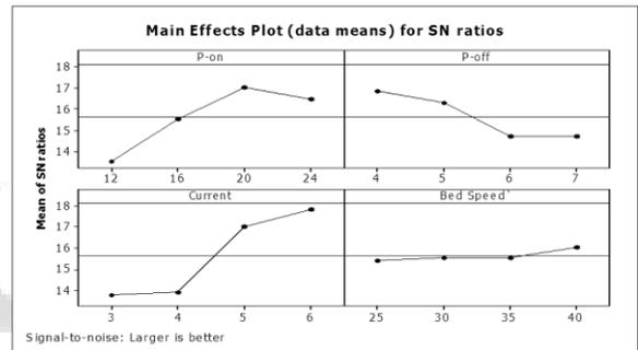
Fig. 11: Effect of Process parameters on MRRv for 20MnCr5 material.
