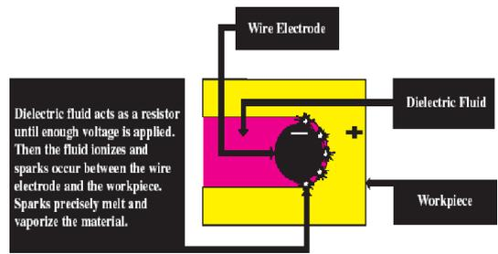
Fig. 4:During in time controlled spark erodes the material
