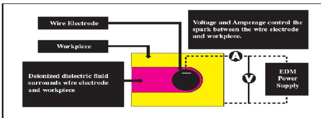
Fig. 3: Power supply generates Volts and amps
