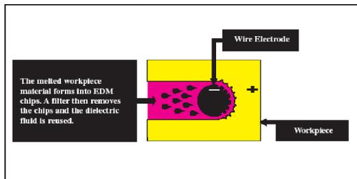
Fig. 6: Filter Removes Chips While the Cycle is repeated
