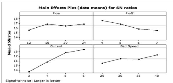
Fig. 10: Effect of Process parameters on MRRv for 16MnCr5 material.
