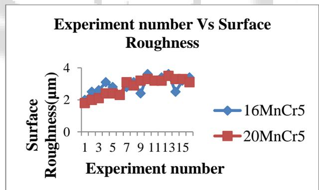
Fig. 8: Comparison of surface roughness for 16MnCr5 and 20MnCr5 materials.
