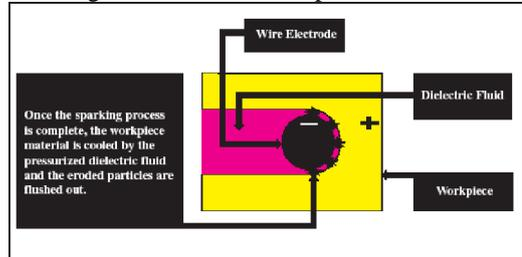
Fig. 5: off Time Allows Fluid to Remove Eroded Particles
