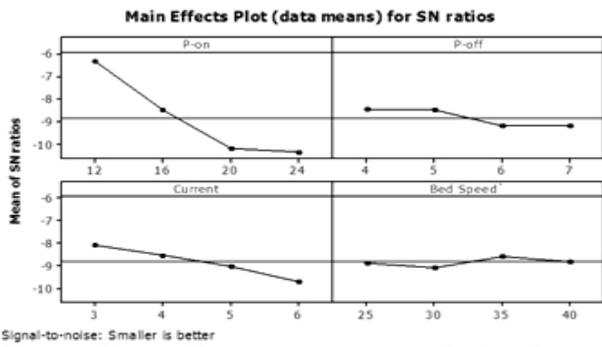
Fig. 14: Effect of Process parameters on Surface Roughness for 20MnCr5 material.
