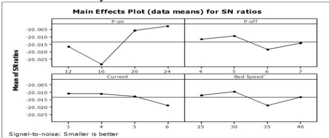
Fig. 12: Effect of Process parameters on Accuracy for 20MnCr5 material.
