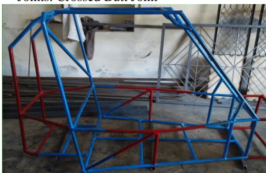
Fig. 5: Fabrication of Roll Cage Structure
