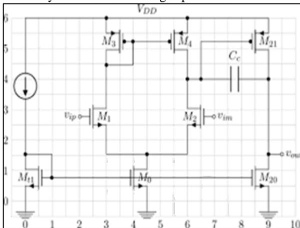
Fig. 2: The topology chosen for this Op-Amp design.
