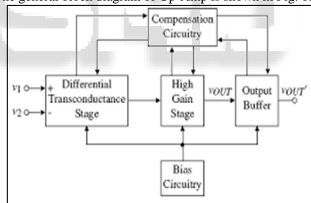
Fig. 1: Block diagram of Op-Amp
