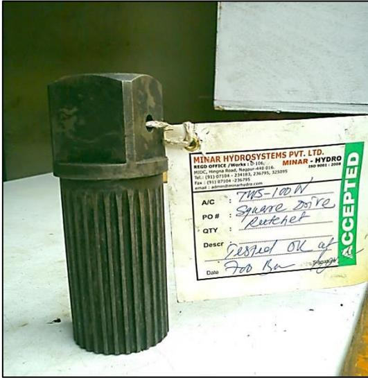
Fig. 4: Drive Adaptor Testing Result Showing It Is Tested at 700 bar Pressure
