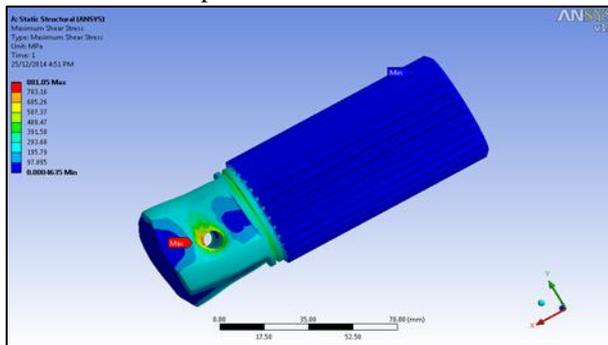
Fig. 2: Static Srtuctural Analysis by Providing Turning Moment to Left End of Adaptor in the ANSYS Software. [2]
