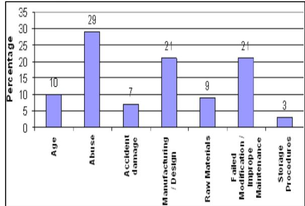
Fig. 1: The Common Causes of Service Failure
