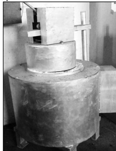
Fig. 3: Furnace for Heat Treatment of Drive Adaptor [7]
