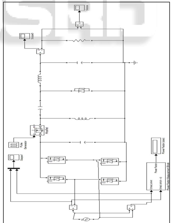
Fig. 14: Simulation Circuit Diagram for Proposed System
