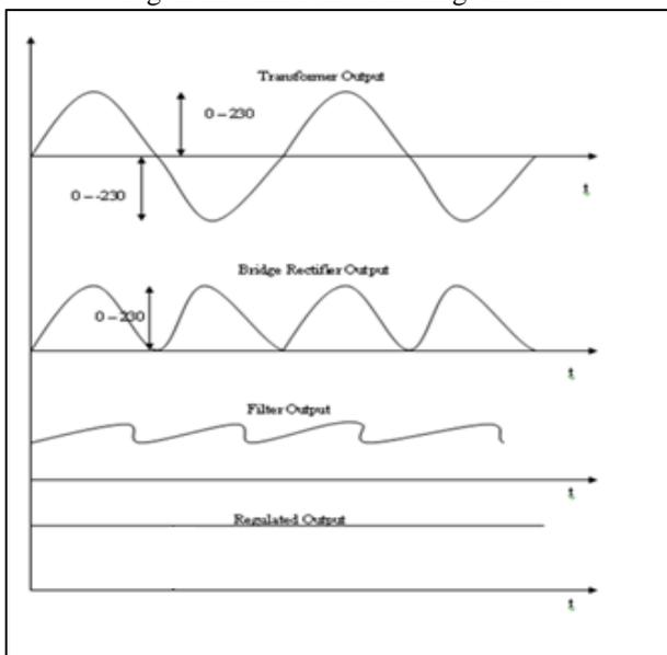
Fig. 3: Wave Form of Regulated Power Supply
