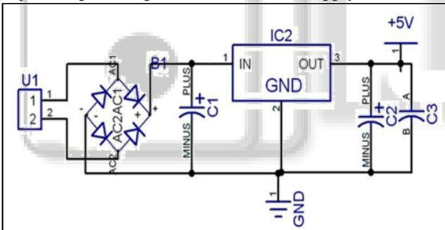
Fig. 2: Rectifier and Filtering Circuit
