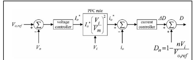
Fig. 8: Control Block Diagram of Proposed Converter
